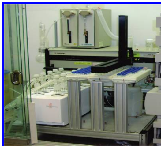
Figure 1. Anachem SK233 platform.
